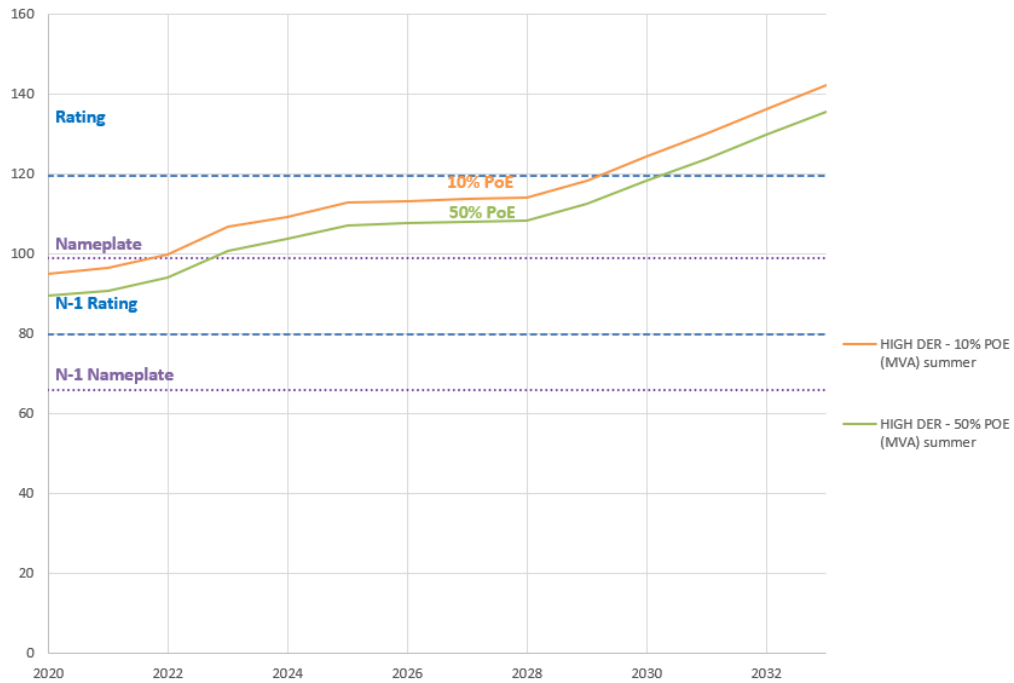
Figure 4 Laverton Substation (LV) Summer Loading Forecast (MVA)
